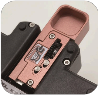
Blade position can be renewed without tools
