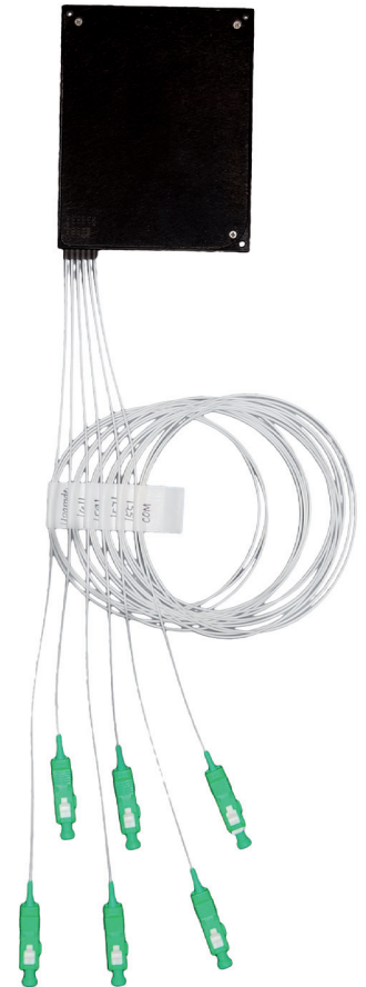
CWDM multiplexer with 900 µm buffered fibre leads
